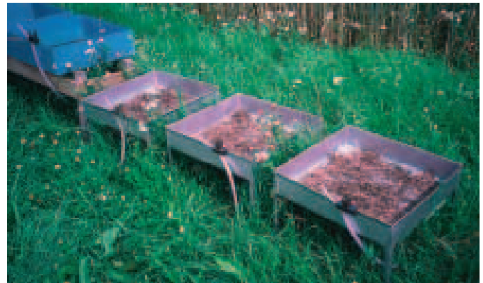
Fig. 1b. In order to measure the leaching losses , precipitation water that passed through the cut plant material was collected, quantified and analysed for total N, P and C content.
