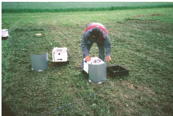
Figure 1. Equipment used for measuring a) ammonia emissions and b) leaching from cut plant material to soil.
