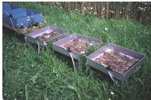
Figure 1. Equipment used for measuring a) ammonia emissions and b) leaching from cut plant material to soil.
