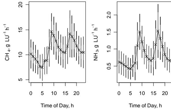
Figure 1. Diurnal variations in the emission rates of CH<sub>4</sub> and NH<sub>3</sub> measured in the dairy cow barn. The crosses in the undulating line represent the hourly averages for the entire sampling period (26<sup>th</sup> Feb–9<sup>th</sup> May, 2008). Vertical lines represent standard deviations.
