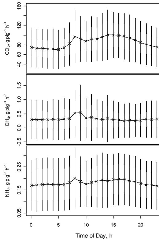
Figure 2. Diurnal variations in the emission rates of CO<sub>2</sub>, CH<sub>4</sub> and NH<sub>3</sub> measured in the piggery in spring. Crosses in the undulating line represent the hourly averages for the entire sampling period (4<sup>th</sup> April–9<sup>th</sup> June, 2007), while the vertical lines represent standard deviations.
