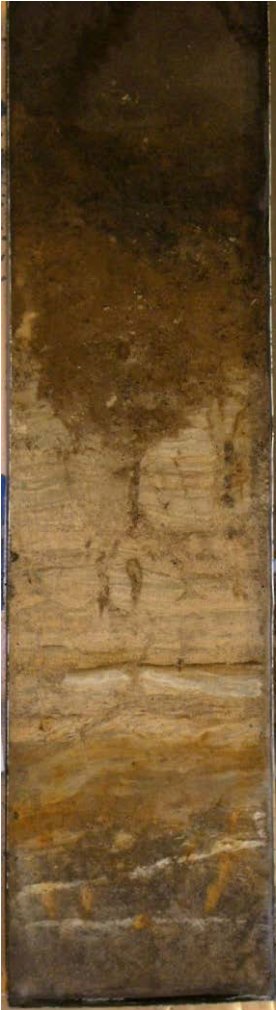
The Mellby soil profile, 0-90 cm depth
